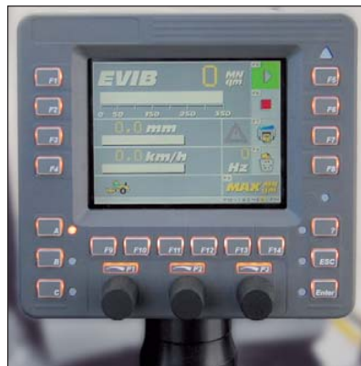
Compaction control systems such as BTM plus show load-bearing results in real-time.
