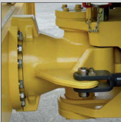
The articulated joint is maintenance-free and so are the travel bearings and the steering cylinders ...
