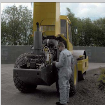
With the hood wide open, excellent access is provided to all components in the engine compartment.
